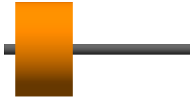
Figure 16: Experimental arrangement reproduced as a beamline in BDSIM. The orange rectangle shows the region occupied by the electric field map with a length of 36 cm. The phosphor screen is placed 67 cm downstream of the Gabor lens.
