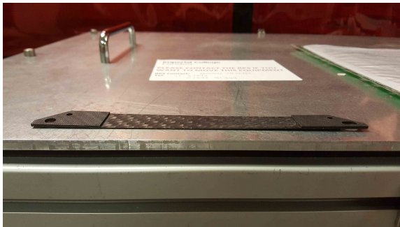
Figure: New prototype of the clear connector which introduces a recess.
