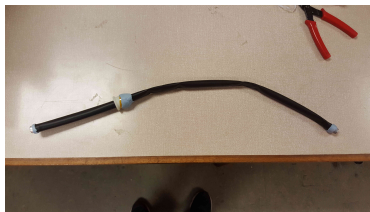
Figure: Bundle of scintillating and clear fibres into heat shrink, ready to be potted.
