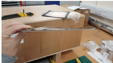
Figure: Second prototype still shows bending along with fibre misalignment after wires cut.
