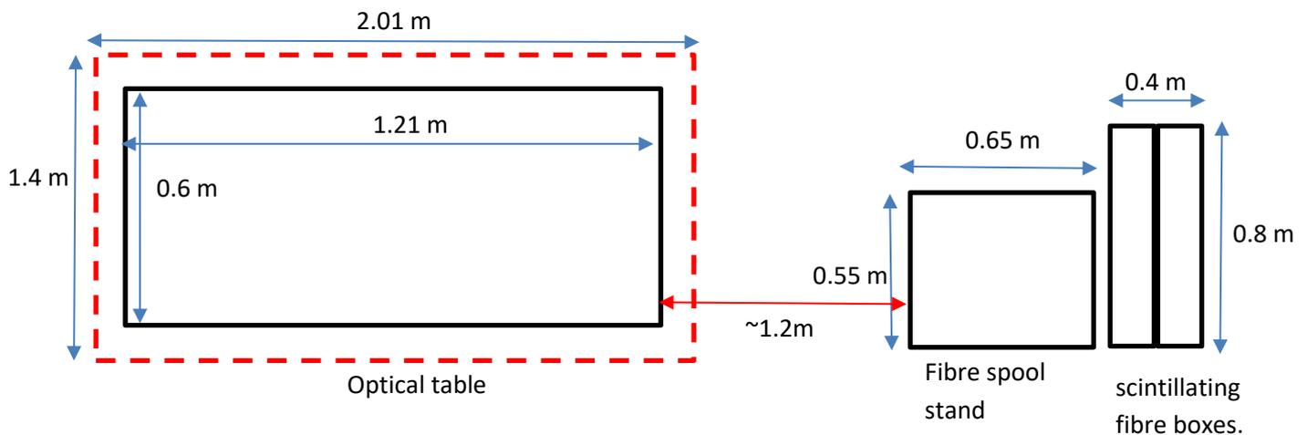
Around the optical table is marked a clearance area. This is ideally 0.4m wide all the way round the table. The distance marked between the fibre spool stand and the optical table is used to allow the fibre to slacken when winding. This is ideally 1-1.5m and can be in the direction marked or perpendicular to the table.
