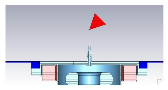
Red triangle is laser beam (because James Bond, Goldfinger) point lands on light blue target Blue is laser vacuum vessel with 2 ISO320 flanges shown.
