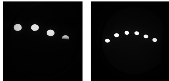
Figure 11: Observed camera image of the 3 beam spots beyond the aperture in the Setup 1 configuration, left, and with 6 beam spots beyond the aperture in the Setup 2 configuration, right. Both images were taken with the lens off
