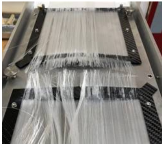
Figure: Tension issues in first prototype.
