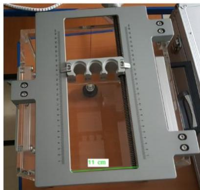
Figure 2: Photographs of a commercially available water phantom.
