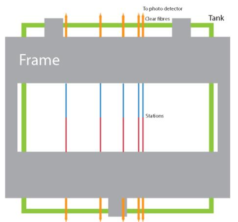
Scintillating-fibre detectors, each 15 x 15 cm<sup>2</sup>.
