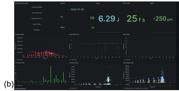
Figure 3: (a) Diagram of the automated data scan control capability. (b) Example image of the Grafana based dashboard system for monitoring source performance.
