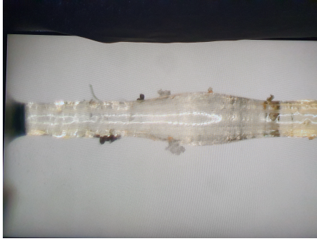
Image of the long length of the fibre. Image shows the end of the length where the fibres had been fitted into the casing.
