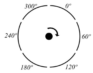
The relative phase of the signal applied to each sector of the electrode is labelled.
