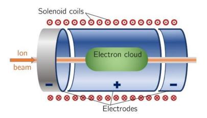
Using the Penning-Malmberg trap, a linear array of electrically biased cylinders arranged along the axis of a uniform magnetic field.
