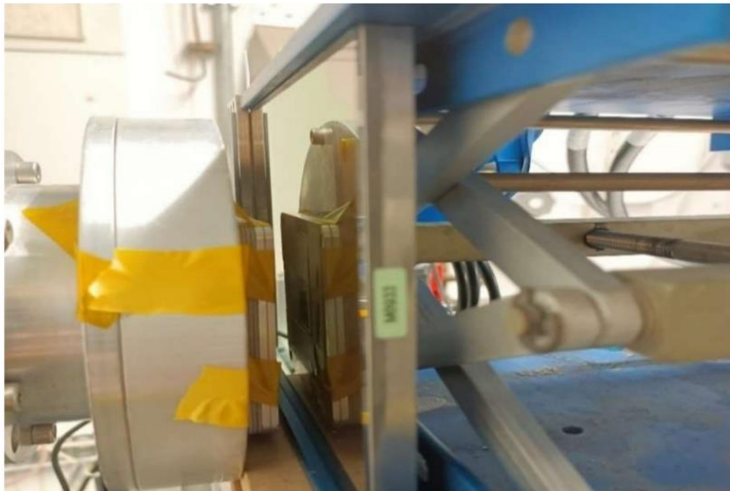
Figure 3.10 – Experimental setup of the air measurements. The reflection of the taped collimator can be noticed in the CMOS.
