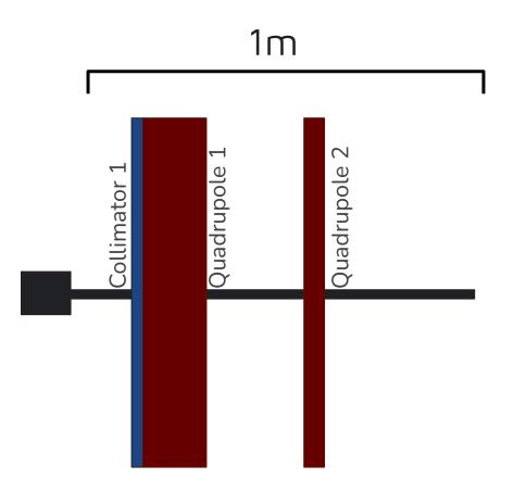
Finding the optimal position of the first quad pair to find the smallest spot size through at 1m
