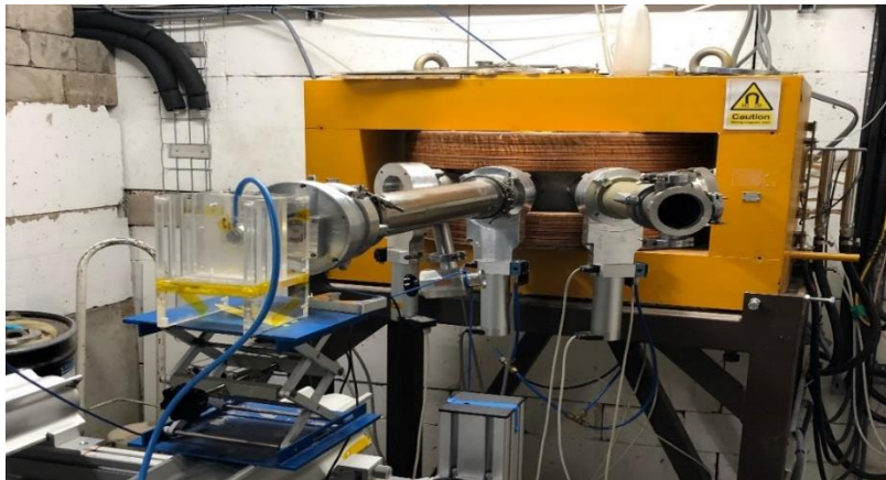
MC-40 cyclotron for particle (proton and helium) ion irradiations, including at FLASH (100 Gy/s) dose rates
