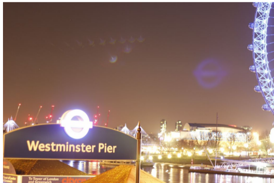
Ghosting due to total internal reflection of bright sources in optical photography
