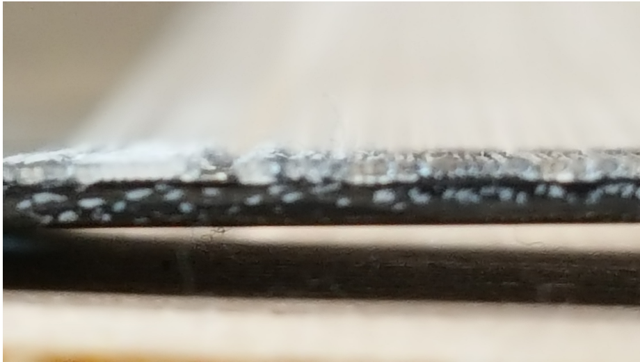
Figure 12: An image of one of the ends used for alignment. There are some noticeable gaps where during the gluing process some of the fibres have shifted to group and stick together.
