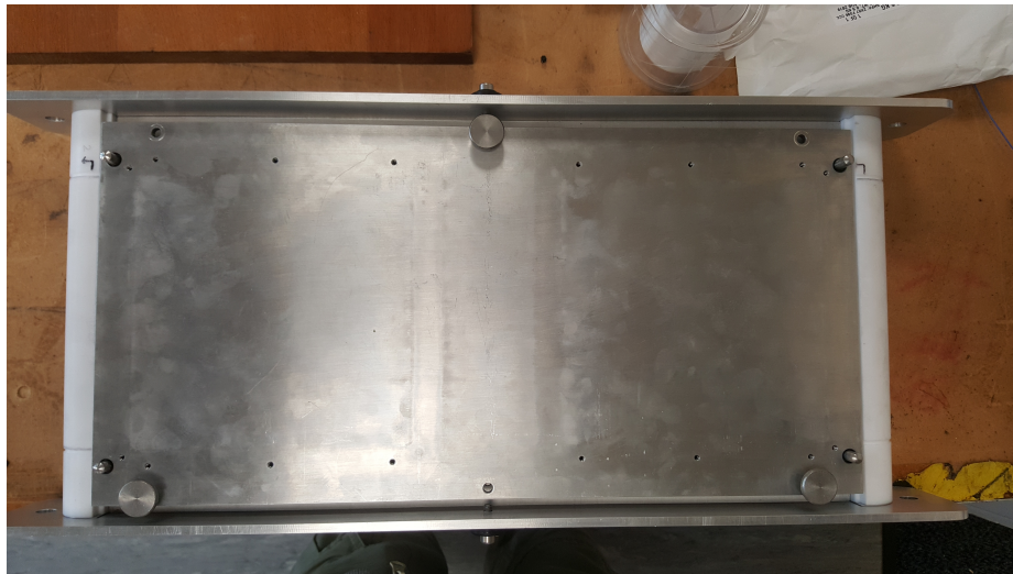
Figure 17: Modifications were made to the winding jig, where the lobes were cut in half length wise and positioned adjacent to the platen to keep the wires from moving when gluing in order to help with the alignment.
