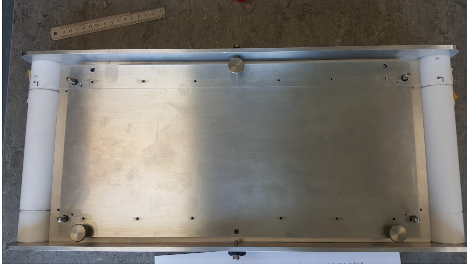
Figure 1: Assembled winding jig with two winds of fishing wire across the two lobes.
