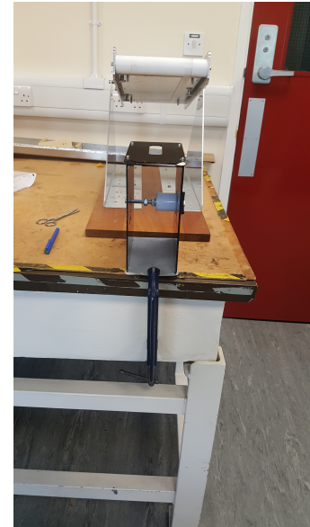
Figure 2: The setup for the winding jig at RAL. On the left one can see the winding jig affixed to the outer frame atop a wooden plank. On the right one can see the tensioning solution, which consists of washers pushing against the spool of fishing wire.
