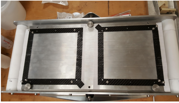
Figure 10: Images of the second prototype after gluing. On the left we see the frames, where with a single layer it is more visually obvious of the wires being glued to the frames. On the right is the connector plates where one side has release film intended to hold the fibres in place while the other side doesn't. It did not appear to help much however.
