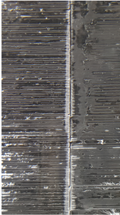
Figure 14: A close up of the connection being made between the frames and connector tab. In the case of the prototype it appears there is a gap which may be an issue of the fishing wire not being polished on the edges.
