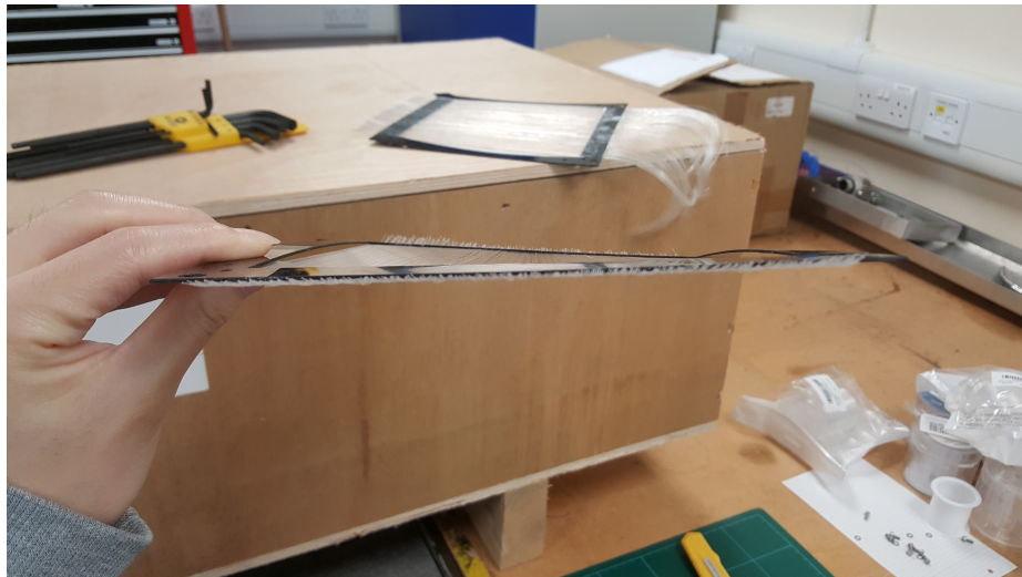
Figure 11: The result of the frame bending after the wires were cut for the second prototype.
