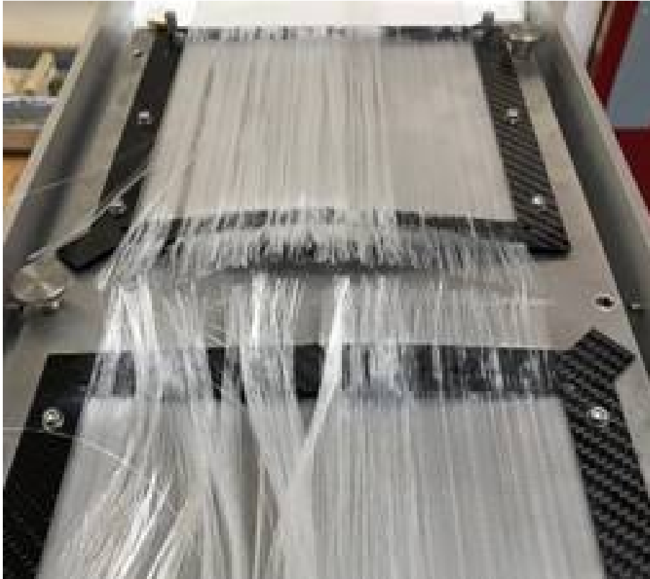
Figure 7: The result after the wires were cut where the tension in the wires caused both frames to bend.
