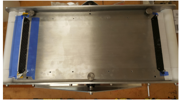
Figure 10: Images of the second prototype after gluing. On the left we see the frames, where with a single layer it is more visually obvious of the wires being glued to the frames. On the right is the connector plates where one side has release film intended to hold the fibres in place while the other side doesn't. It did not appear to help much however.
