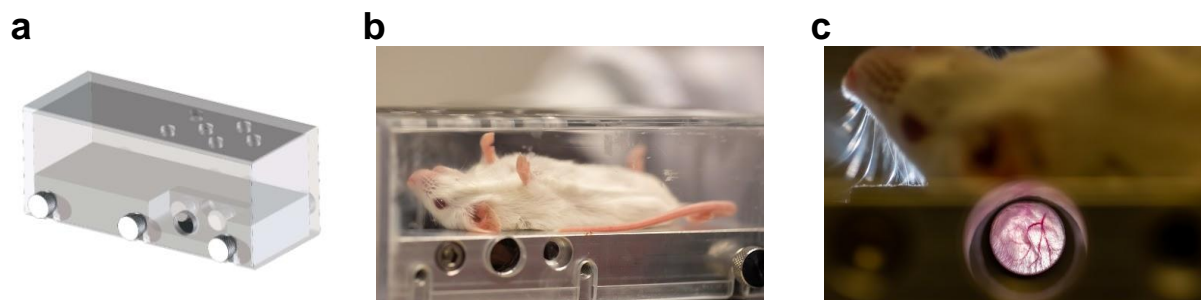
Figure 6. Mouse ear irradiation assembly. a Design of the assembly with ear clamp, aluminum base and plexiglass top with breathing holes. b Photographs of the mouse holder with anesthetized mouse and clearing for the proton beam path during irradiation campaign at the BELLA PW proton beamline. c Close-up of the proton beam path and mouse ear, showing vascular structure.
